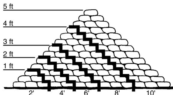
Estimated cubic yards of sand needed per 100 feet of dike length for various dike heights and ratios of height to width. An additional 2 cubic yards will be needed for bags to hold the plastic.
