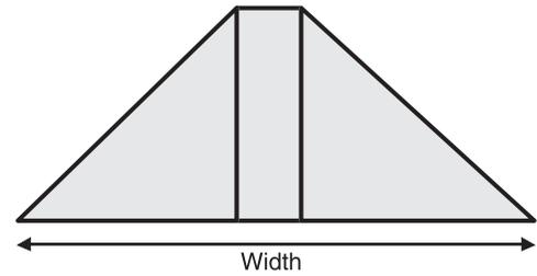
This volume is calculated based on a center section that is 9 inches wide and the remainder is in a triangular shape.
